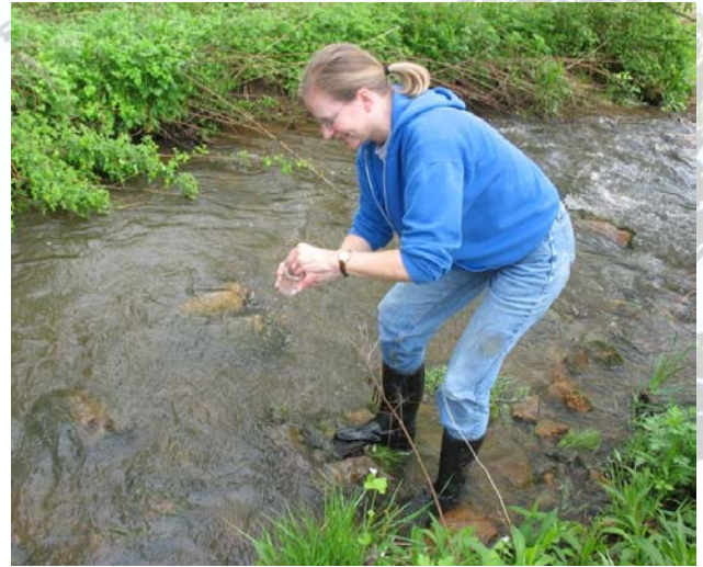
Rutgers Cooperative Extension Water Resources Program Associate collecting water quality sample sfor fecal coliform bacteria analysis along a tributary to Musconetcong River in Warren County
