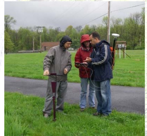
Project Team members in the Rockaway Creek Watershed collect field data (soil moisture) to verify modeling results . May 2009
